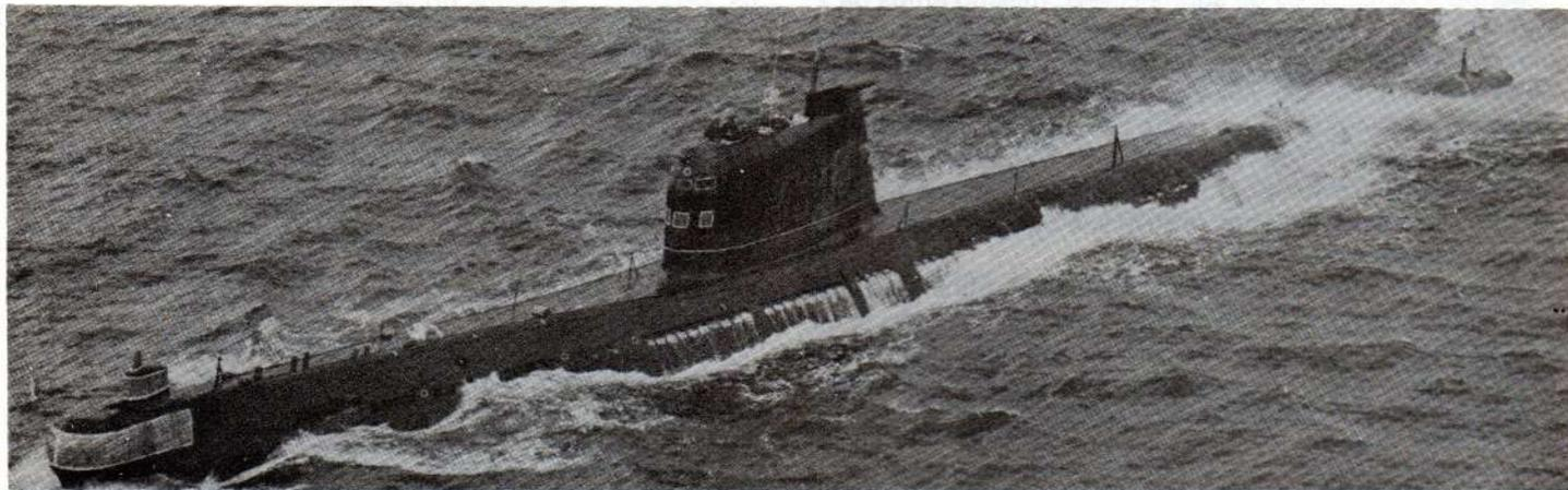
Foxtrot-class SS in the Pacific. These are considered efficient, long-range patrol submarines. (1984, JMSDF)
